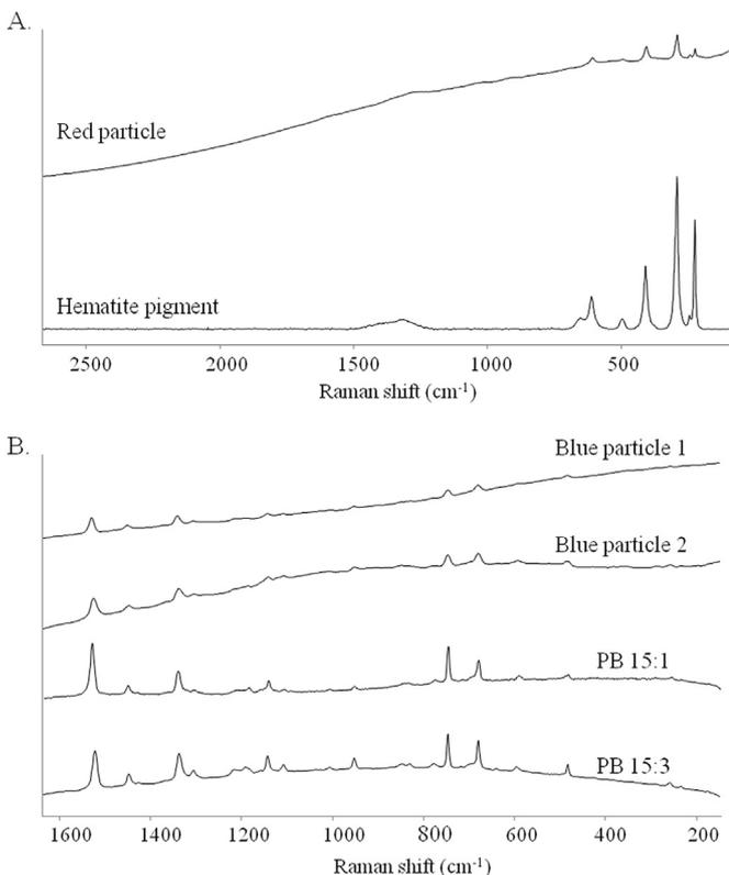
**Fig. 3.** Identification of microparticles using micro-Raman spectroscopy. A. The Raman spectrum of a red particle extracted from *M. edulis* tissue corresponds to that of the pigment haematite. B. The Raman spectra of two blue particles (particle 1 from *C. gigas* and particle 2 from *M. edulis*) correspond to that of the widely used phthalocyanine dyes PB 15:1 and PB 15:2, respectively.
